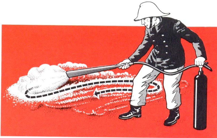
Fig. 7.3 Method of operating a \text{CO}_2 extinguisher by sweeping the discharge horn across the surface of the burning material.
